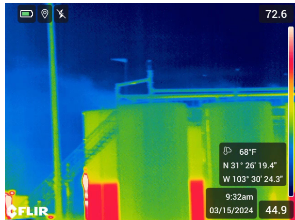
Using Optical Gas Imaging (OGI) technology, Oilfield Witness is able to visualize and record otherwise invisible methane plumes. In this case the plume is arising from a series of storage tanks.
